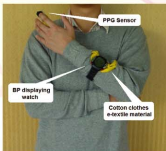
Frontal view of the h-Shirt and blood pressure displaying watch 保健衫(h-Shirt)的外觀及血壓顯示表
