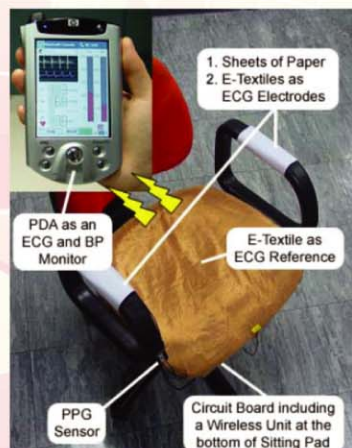
Design of a blood pressure monitoring chair. 血壓監測坐椅的設計
