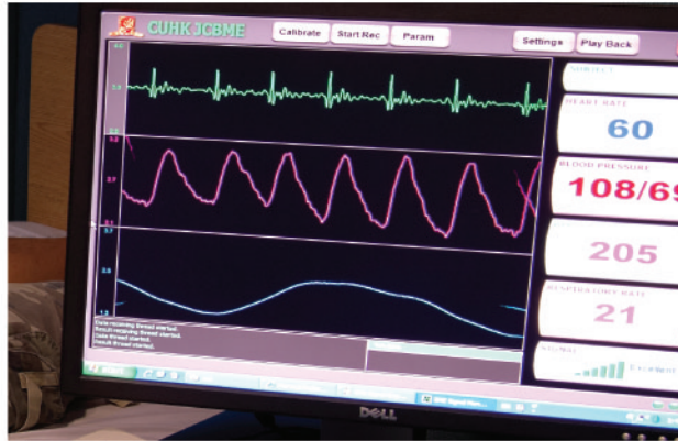
The monitoring system can display heart rate, blood pressure and respiration rate 監測系統能同時顯示心率、血壓及呼吸率
