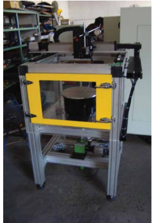
Fabricated mechanism for magnetorheological jet finishing of optical elements 構建的磁流液噴射光學元件拋光機
