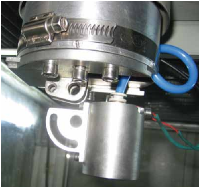
Specially designed nozzle for formation of magnetorheological jet 特別設計的磁流液射噴嘴以達致噴射效果
