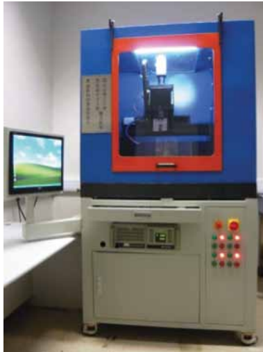
Constructed MR fluid polishing machine 設計和構建的磁流液輔助拋光機
