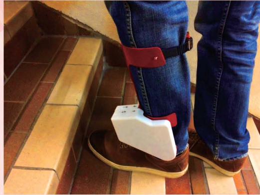
Stroke patient walks upstairs and downstairs with the ankle robot 中風患者使用機械腳托上落樓梯
