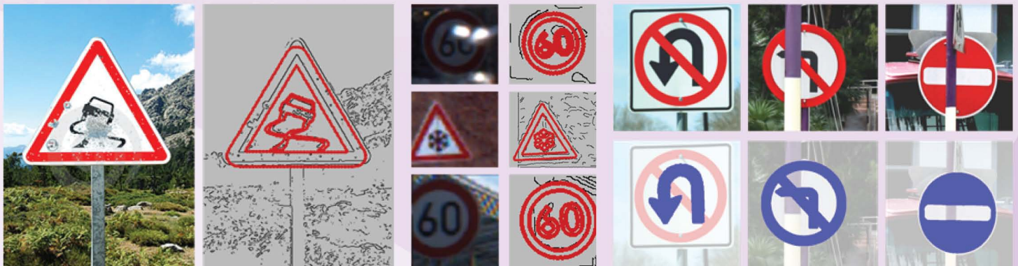
The system can successfully recognize the traffic signs even under the partial occlusion attack and other harsh conditions. 系統在有局部遮擋或其他惡劣的情況下仍能成功識別出路標。
