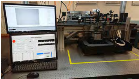
SLD prototype (including software, optical system and motion system) 隱形激光切割系統原型 (包括軟件、光學和運作系統)
