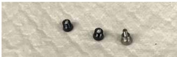
The screw with new design did not break off, compared to previous design, after the screws were completely inserted into the tibia of goat
