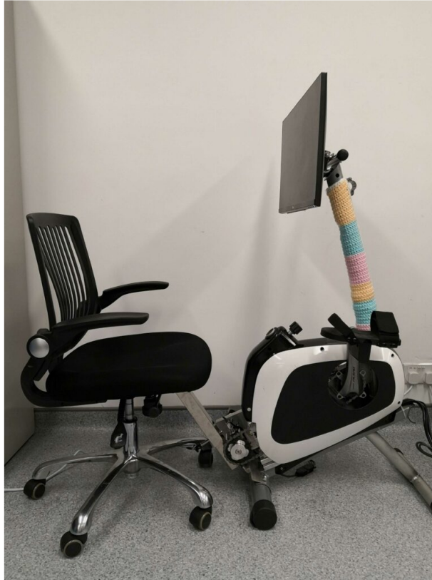
Neuro-Muscular Electrical Stimulation (NMES) motor-assisted cycling system
