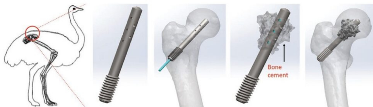
Mg-based stent with holes in the shaft for injection of bone cement to repair osteonecrosis in the femoral head in emu
